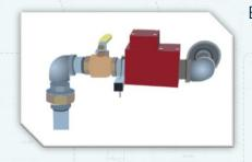
By far the most cost-effective means to mitigate or prevent a damage from a natural gas accident is installing seismic shut-off valves. In the event of an earthquake, these will stop gas flow on a premises and preclude a fire from igniting – from any number of ignition sources (electrical lines, sparks, open flames, pilot lights, etc.) downstream on the gas line. Typically,
